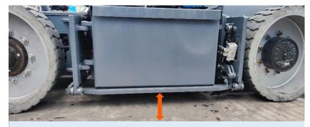
**Automatic pothole protection device** will be extended when boom is lifting and retracted when boom is lowering.
