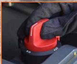
Battery cut-off switch
