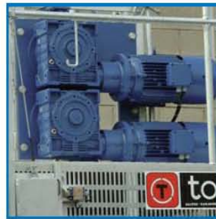
Grupo motriz: motorreductores con electrofreno integrado Drive unit: gearmotors with built-in electric brake
