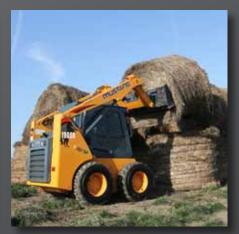
operate safely with clear side and rear sight lines for full, expansive views for increased safety and precision placement. A roof grid section provides visibility to the bucket at full lift height.
