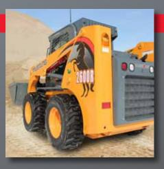
SMOOTH RIDE ▲ is achieved with a longer wheelbase and low center-of-gravity. The HydraGlide<sup>™</sup> ride control option provides stable operation over uneven surfaces.
