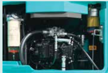
Fuel filter with built-in water-separator
