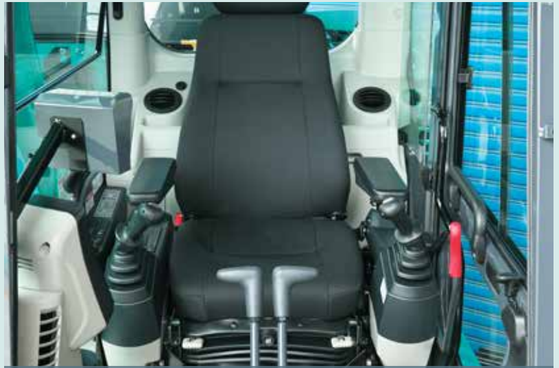
Seat suspension absorbs vibration
