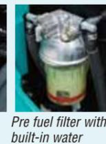
Pre fuel filter with built-in water separator
