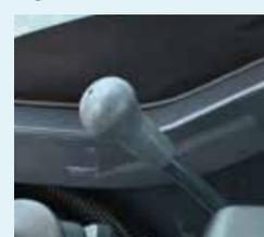
The dozer lever features hydraulic pilot control for precise handling.
