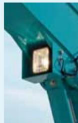
Work lights have been added on both sides to provide a clear view during nighttime operations.
